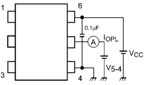
Fig. 13.1.2 I<sub>OPL</sub> Test Circuit
