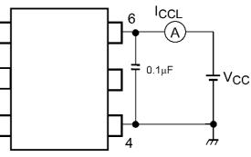
Fig. 13.1.6 I<sub>CCL</sub> Test Circuit
