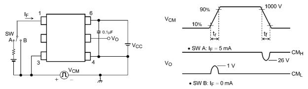
Fig. 13.1.8 Common-Mode Transient Immunity Test Circuit and Waveform
