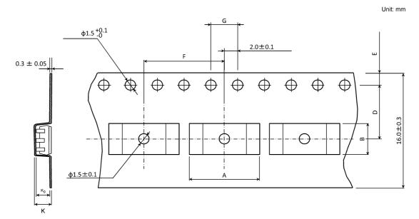
Table Tape Dimensions (unit: mm, tolerance: ±0.1)
