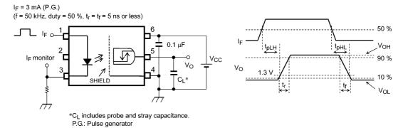
Fig. 13.1.7 Switching Time Test Circuit and Waveform
