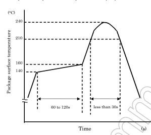
This profile is based on the device's maximum heat resistance guaranteed value.
