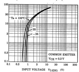
Fig. 10.6 RN1406 I<sub>C</sub>-V<sub>I(ON)</sub>
