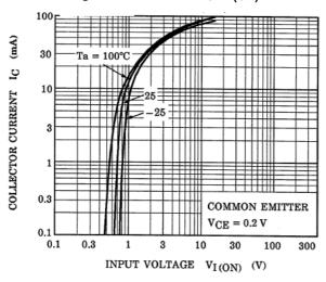
Fig. 10.5 RN1405 I<sub>C</sub>-V<sub>I(ON)</sub>
