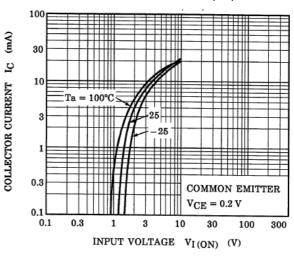
Fig. 10.4 RN1404 I<sub>C</sub>-V<sub>I(ON)</sub>
