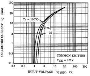
Fig. 10.3 RN1403 I<sub>C</sub>-V<sub>I(ON)</sub>
